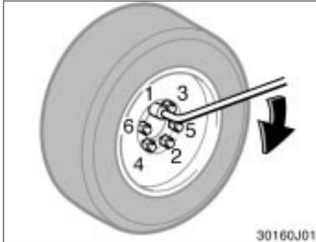
**9. Lower the vehicle completely and tighten the wheel nuts.**
