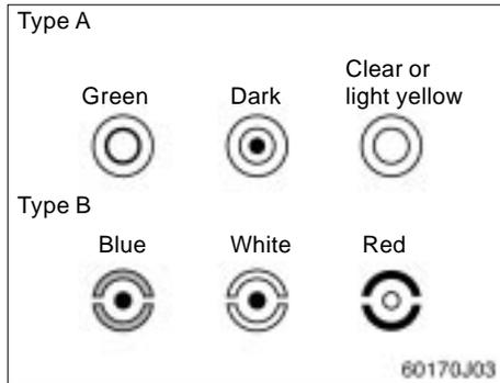
**CHECKING BY THE HYDROMETER**
