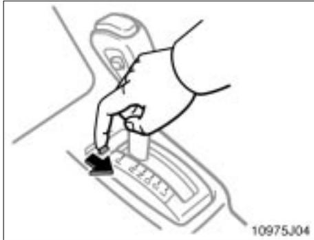
3. Insert your finger into the hole to move the shift lock overdrive lever backward. You can shift out of "P" position only while holding back the lever.
