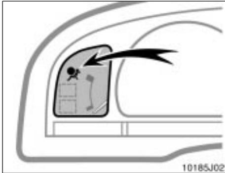
**This indicator comes on when the ignition key is turned to the "ACC" or "ON" position. It goes off after about 6 seconds. This means the SRS airbags are operating properly.**
