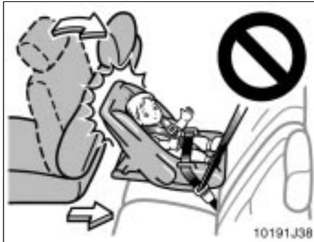
▶ Do not put a rear-facing child restraint system in the rear seat if it interferes with the lock mechanism of the front seats. This can cause severe injury to the child and front passenger in case of sudden braking or a collision.
