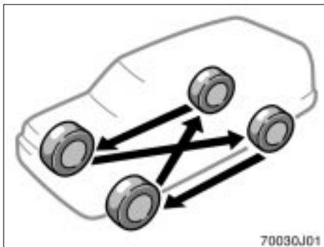
To equalize tire wear and help extend tire life, Toyota recommends that you rotate your tires approximately every 12000 km (7500 miles). However, the most appropriate timing for tire rotation may vary according to your driving habits and road surface conditions.
