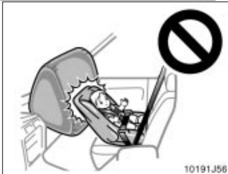
▶ Never put a rear-facing child restraint system in the front seat because the force of the rapid inflation of the passenger airbag can cause death or serious injury to the child.
