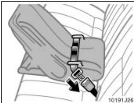
1. Run the center lap belt through or around the infant seat following the instructions provided by its manufacturer and insert the tab into the buckle taking care not to twist the lap belt.
