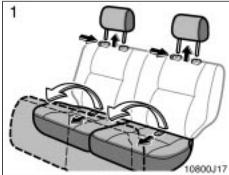
1. Remove the head restraint, and swing the bottom cushion up by pulling the lock release strap. Be certain to replace the head restraint.
