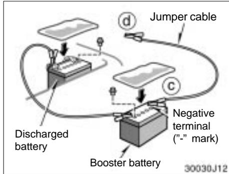
c. Connect the clamp of the negative (black) jumper cable to the negative (-) terminal on the booster battery.
