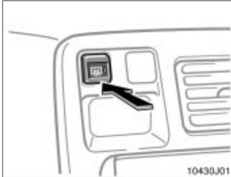
**To defog or defrost the back window, push the switch.**
