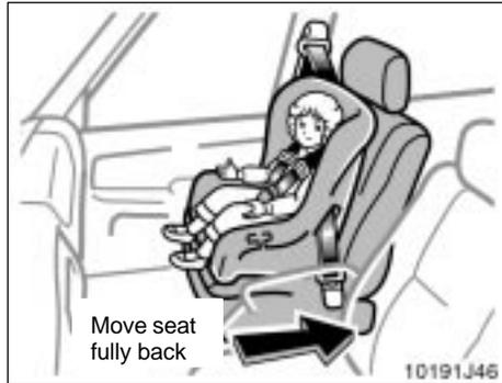
► A forward-facing child restraint system should be allowed to put on the front seat only when it is unavoidable. Always move the seat as far back as possible, because the force of a deploying airbag could cause death or serious injury to the child.
