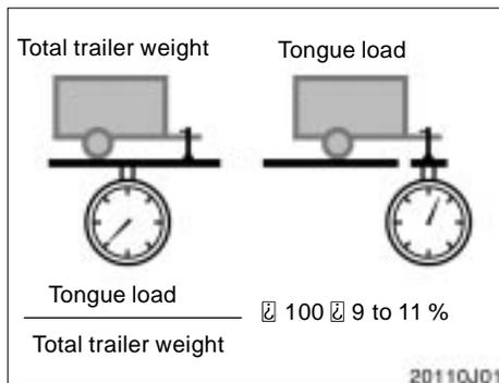
▶ The trailer cargo load should be distributed so that the tongue load is 9 to 11% of the total trailer weight, not exceeding the maximum of the following. Never load the trailer with more weight in the back than in the front. About 60% of the trailer load should be in the front half of the trailer and the remaining 40% in the rear.
