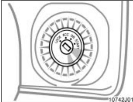
For easy access to the ignition switch, the ignition switch light comes on when the driver's door is opened.
