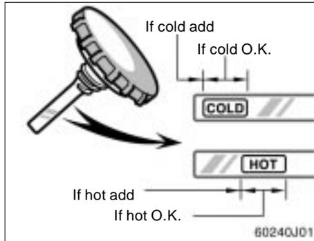
**Check the fluid level on the dipstick. If necessary, add automatic transmission fluid DEXRON®II or III.**
