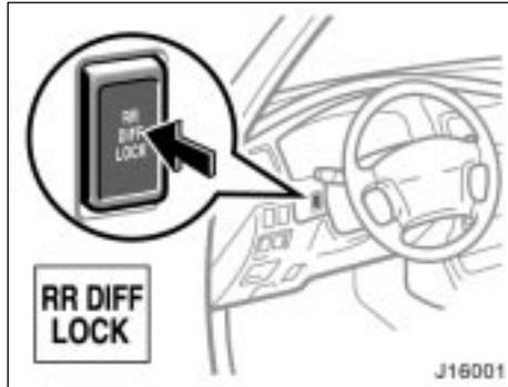
**To lock the rear differential, push the switch.**
