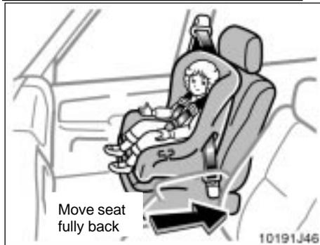
▶ A forward-facing child restraint system should be allowed to put on the front seat only when it is unavoidable. Always move the seat as far back as possible, because the force of a deploying airbag could cause death or serious injury to the child. For instructions concerning the installation of a child restraint system, see "Child restraint" in this chapter.
