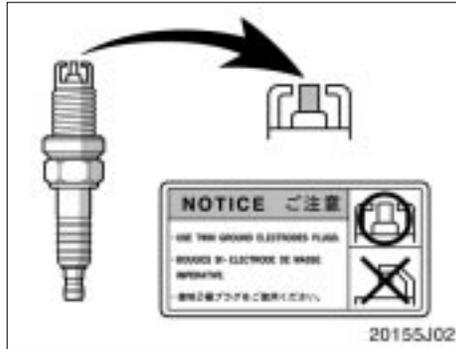
Your engine is fitted with twin ground electrode spark plugs.
