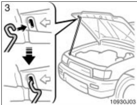
3. Hold the hood open by inserting the support rod into the slot.
