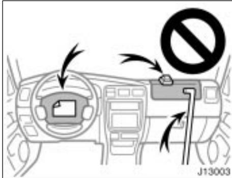
▶ Do not put objects or your pets on or in front of the dashboard or steering wheel pad that houses the airbag system. They might restrict inflation or cause death or serious injury as they are projected rearward by the force of deploying airbags. Likewise, the driver and front passenger should not hold things in their arms or on their knees.
