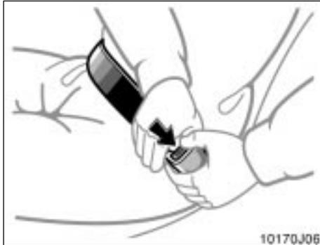
To release the belt, press the buckle-release button. —Stowing rear seat belts
