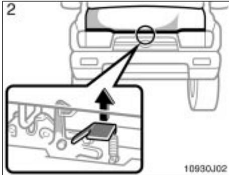
2. In front of the vehicle, pull up on the auxiliary catch lever and lift the hood.
