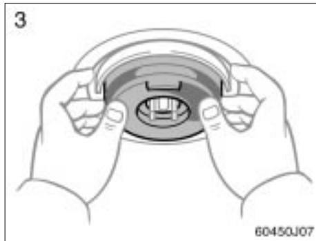
3. Install the rubber cover, and snuggle on the boss. Insert the connector.
