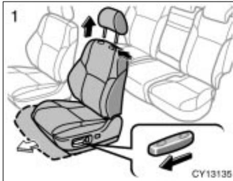
1. Remove the head restraint. Push the seat position adjusting switch forward to slide the seat further forward than the front-most position.
