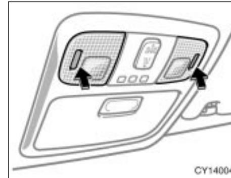
**To turn on the personal lights, push the lens. To turn the lights off, push the lens once again.**
