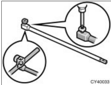
When connecting a jack handle extension with jack handle end, use a Phillips-head screwdriver or jack handle to tighten the bolts on the joints as shown in the illustration.
