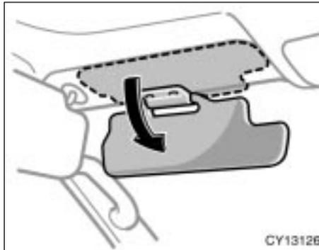
To block the glare from the front when the main sun visor is swung to the lateral side, swing down the sub visor.
