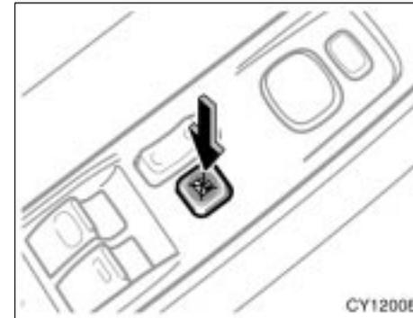
If you push in the window lock switch on the driver's door, the back window cannot be operated.
