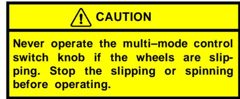
**SHIFTING BETWEEN "H4" (UNLOCKED) AND "H4" (LOCKED)**
