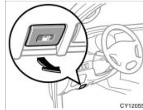
1. To open the fuel filler door, pull the lever.
