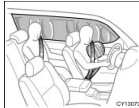
The SRS (Supplemental Restraint System) side airbags and curtain shield airbags are designed to provide further protection for the driver, front passenger and rear outside passengers in addition to the primary safety protection provided by the seat belts.
