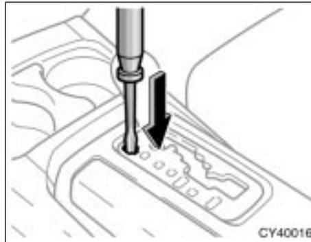
3. Insert the screwdriver or equivalent into the hole to push down the shift lock override button. You can shift out of "P" position only while pushing the button.
