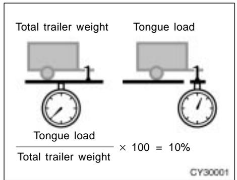
► The trailer cargo load should be distributed so that the tongue load is 10% of the total trailer weight, not exceeding the maximum load of the following.
