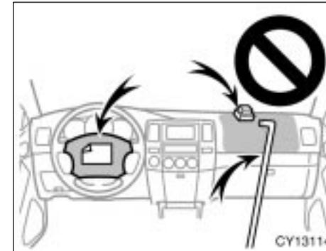
▶ Do not put objects or your pets on or in front of the dashboard or steering wheel pad that houses the front airbag system. They might restrict inflation or cause death or serious injury as they are projected rearward by the force of the deploying airbags. Likewise, the driver and front passenger should not hold objects in their arms or on their knees.
