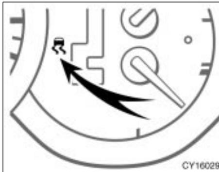
When the hill-start assist control system is operating, the slip indicator light flashes and an alarm sounds intermittently. At the same time, the stop lamps and high mounted stoplight are lit.
