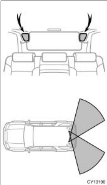
Rear side-view mirrors are useful as a secondary means of checking the area to the rear of the vehicle.
