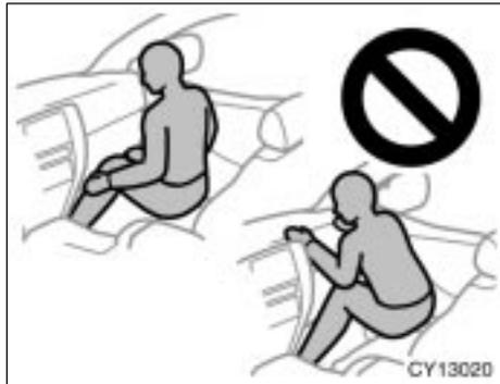
▶ Do not sit on the edge of the seat or lean over the dashboard when the vehicle is in use, since the front airbags inflate with considerable speed and force. Otherwise you may be killed or seriously injured. Sit up straight and well back in the seat, and always use your seat belt properly.
