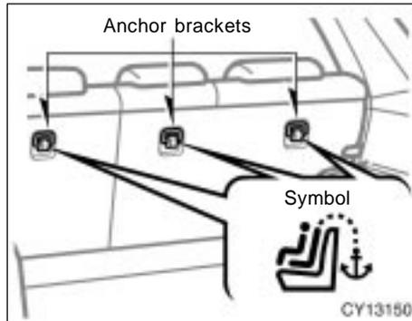
Use the anchor brackets behind the rear seatbacks to attach the top strap. Anchor brackets are installed for each rear seating position. This symbol indicates the location of the anchor brackets.
