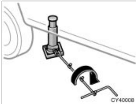
**7. Raise the vehicle high enough so that the spare tire can be installed.**
