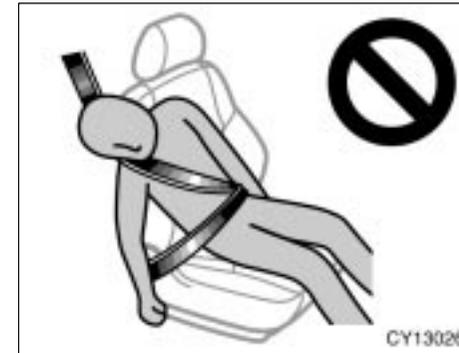
▶ Do not lean against the door when the vehicle is in use, since the side airbag and curtain shield airbag inflate with considerable speed and force. Otherwise, you may be killed or seriously injured. Special care should be taken especially when you have a small child in the vehicle.
