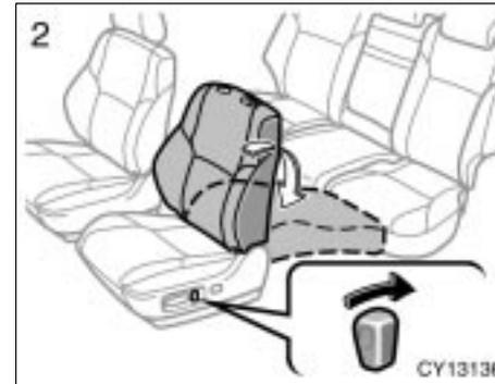
2. Move the seatback angle adjusting switch backward to flatten the seatback.
