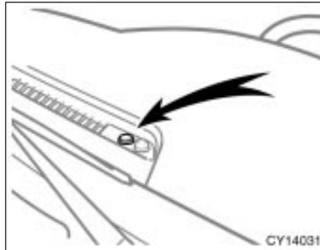
The automatic light control sensor is on the top of the driver's side instrument panel.
