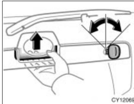
**To open the back door, pull up the back door opener.**
