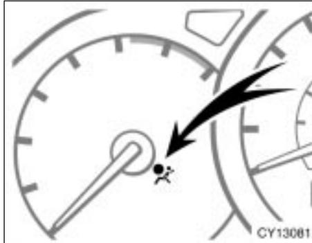
This front seat belt pretensioner system has a service reminder indicator to inform the driver of operating problems. If any of the following conditions occurs, this indicates a malfunction of the airbags or pretensioners. Contact your Toyota dealer as soon as possible to service the vehicle.
