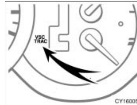
**If there is any abnormality in the system, the "VSC TRAC" warning light will come on. When the "DAC" switch is pushed, the downhill assist control system indicator light also flash.**
