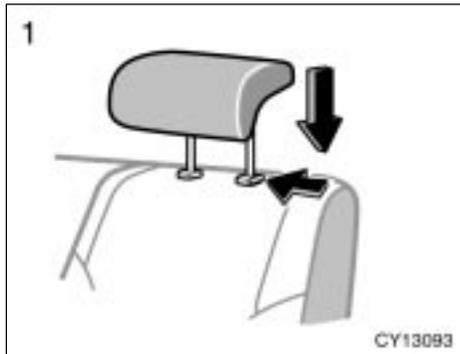
**1. Lower the head restraint to the lowest position.**
