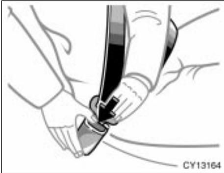
**To release the belt, press the buckle-release button and allow the belt to retract.**
