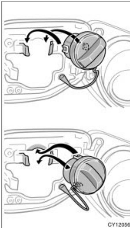
3. The removed cap can be stored on the back side of the fuel filler door.
