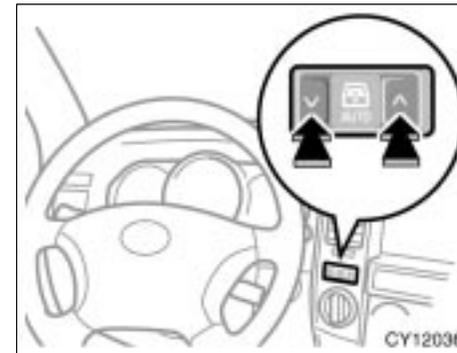
The back window can be operated with the switch on the instrument panel or the key operation in the back door key-hole.
