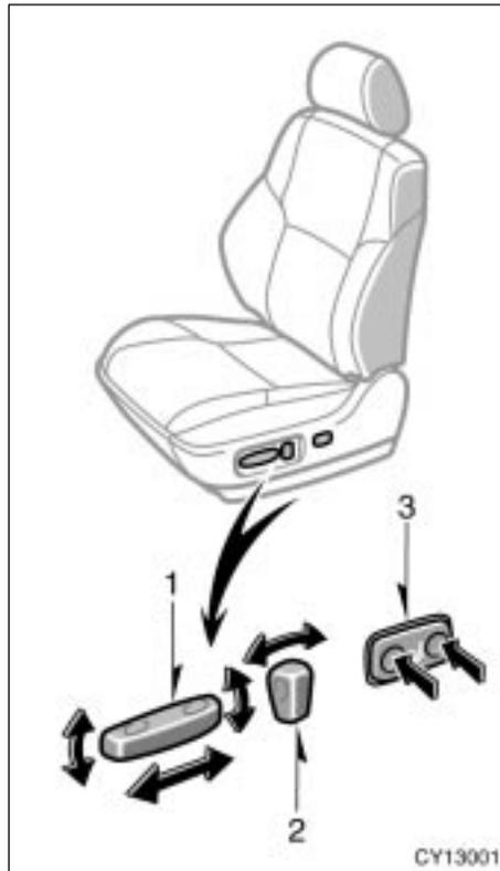
**1. DRIVER'S SEAT: SEAT POSITION, SEAT CUSHION ANGLE AND SEAT HEIGHT ADJUSTING SWITCH**
