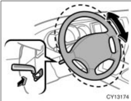
To change the steering wheel angle, hold the steering wheel, pull the lock release lever toward you, tilt the steering wheel to the desired angle and release the lever.
