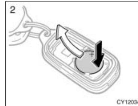
2. Remove the discharged transmitter battery.
