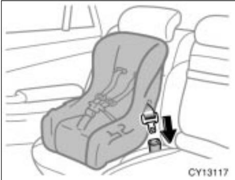
▶ Do not install a child restraint system on the rear seat if it interferes with the lock mechanism of the front seats. This can cause death or serious injury to the child and front passenger in case of sudden braking or a collision.
