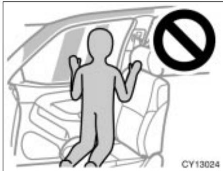
▶ Do not allow a child to kneel on the passenger seat facing the passenger's side door, since the side airbag and curtain shield airbag inflate with considerable speed and force. Otherwise, the child may be killed or seriously injured.
