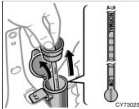
If any washer does not work, the washer tank may be empty. Check the washer fluid level on the level gauge. If the washer fluid level is below "LOW" or only slightly above the "LOW" level, add washer fluid.
