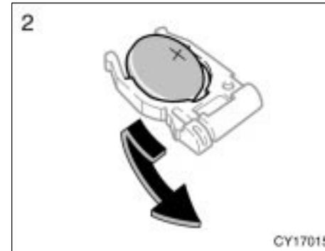
2. Remove the discharged battery.
