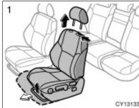
1. Remove the head restraint. Hold the center of the lever and pull it up. Then slide the seat further forward than the front-most lock position.
