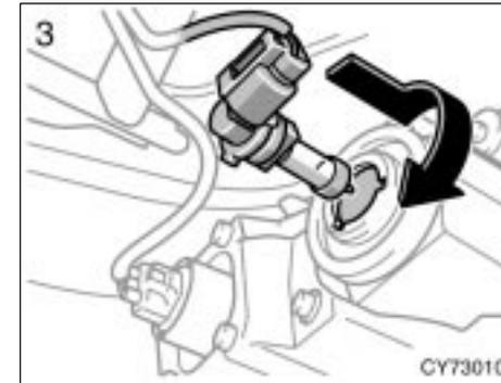
3. Install a new bulb and connector into the mounting hole and turn them clockwise to the front of the vehicle.
