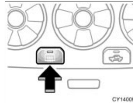
To defog or defrost the back window, push the switch with the back window closed.
