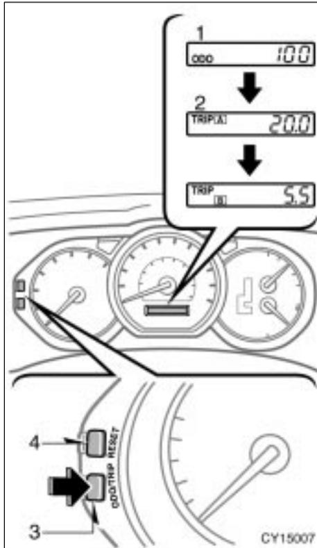
**This meter displays the odometer and two trip meters.**
