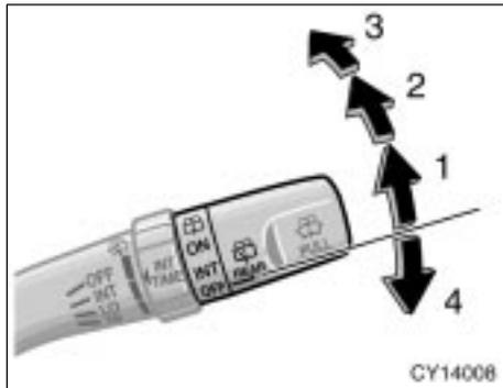
If the back window is not fully closed, the back window wiper and washer will not work. Make sure the back window is fully closed when using the back window wiper and washer.
