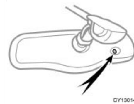
To ensure correct functioning of an anti-glare mirror sensor located on the back side of the mirror, do not touch or cover the sensor with your finger or a piece of cloth, etc.
