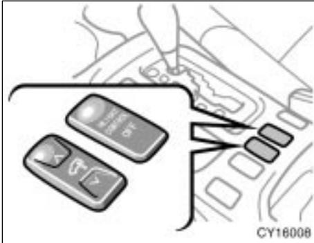
This rear height control air suspension controls the vehicle height depending on the vehicle driving conditions. Select your desired height among the “HI” (high), “N” (normal) and “LO” (low) modes with the height select switch.
