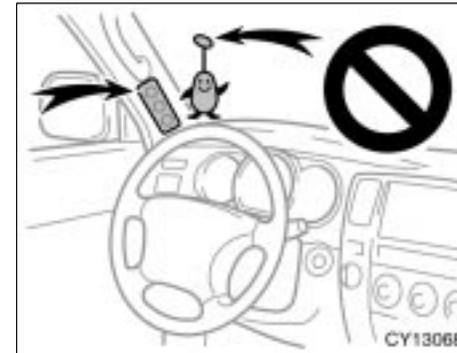
▶ Do not attach a microphone or any other device or object around the part where the curtain shield airbag activates such as on the windshield glass, side door glass, front and side pillars, roof side and assist grips. When the curtain shield airbag inflates, the microphone or other device or object will be thrown with great force or the curtain shield airbag may not activate correctly, resulting in death or serious injury.
