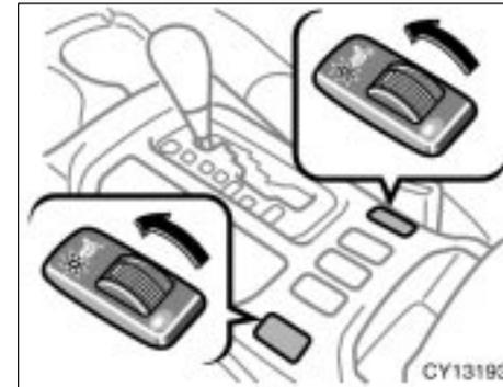
**To turn on the seat heater, move the dial forward (“L” dial for the left front seat and “R” dial for the right front seat). At this time, the indicator light will illuminate to indicate the seat heater is operating.**
