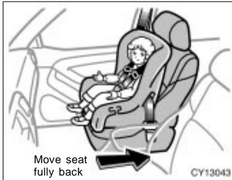
▶ A forward-facing child restraint system should be allowed to be installed on the front passenger seat only when it is unavoidable. Always move the seat as far back as possible, because the force of the deploying front passenger airbag could cause death or serious injury to the child.
