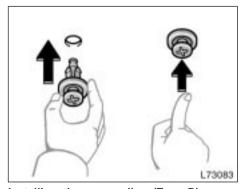
Installing the cover clips (Type B)
