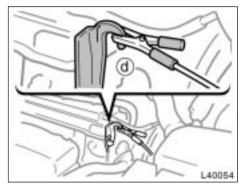
Connecting point for 5S-FE engine
