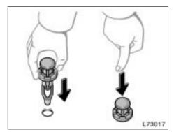
Installing the cover clips
