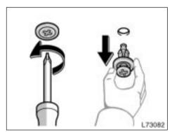
Removing the cover clips (Type B)
