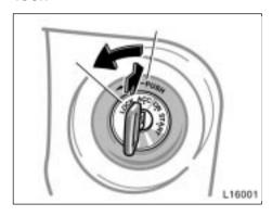
"START"—Starter motor on. The key will return to the "ON" position when released.
