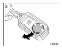
Remove the discharged transmitter battery.
