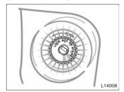
For easy access to the ignition switch, the ignition switch light comes on when any of the doors are opened.
