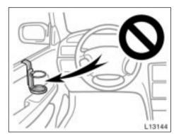
Do not attach a cup holder or any other device or object on or around the door. When the side airbag inflates, the cup holder or any other device or object will be thrown with great force or the side airbag may not activate correctly, resulting in death or serious injury. Likewise, the driver and front passenger should not hold things in their arms or on their knees.
