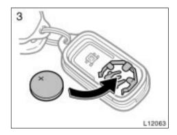
3. Put new transmitter battery with positive (+) side up.
