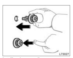
Installing the cover clips
