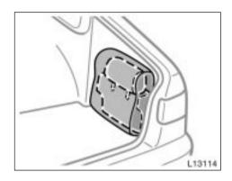
Insert the head restraint and upper pad into the storage bag. Then place the storage bag into the trunk by attaching with Velcro.
