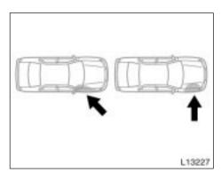
The SRS side airbag system may not inflate if the vehicle is subjected to a collision from the side at certain angles, or a collision to the side of the vehicle body other than the passenger compartment as shown in the illustration.
