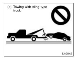
(c) Towing with sling type truck
