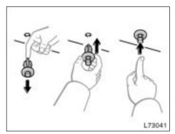
Installing the cover clips (Type A)
