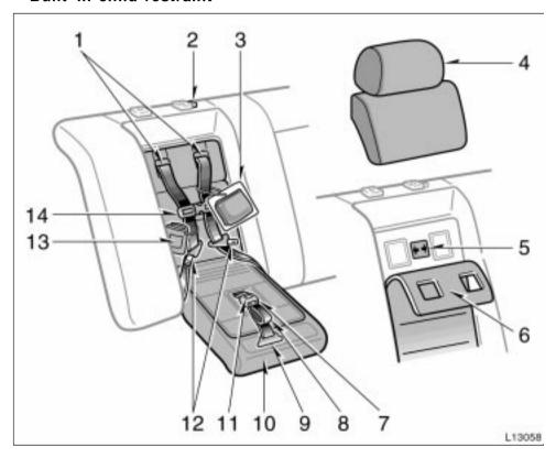
The built-in child restraint system mainly consists of a child seat integrated in the rear seat and 5-point seat belts. Refer to the illustration to become familiar with the parts of the system. This child restraint system conforms to U.S. Motor Vehicle Safety Standard No.213 and Canada Motor Vehicle Safety Standard No.213.4.
