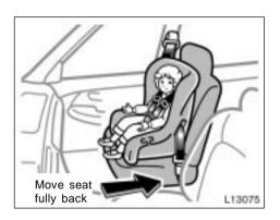
A forward-facing child restraint system should be allowed to be put on the front seat only when it is unavoidable. Always move the seat as far back as possible, because the force of a deploying airbag could cause death or serious injury to the child. Do not allow the child to lean against the front door or around the front door even if the child is seated in the child restraint system. It is dangerous if the side airbag inflates, and the impact could cause death or serious injury to the child.
