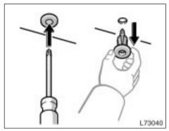
Removing the cover clips (Type A)
