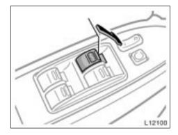
Automatic operation (to open only): Push the switch completely down and then release it. The window will fully open. To stop the window partway, lightly pull the switch up and then release it.
