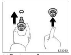
Installing the cover clips
