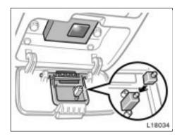
If the center panel does not contact with your garage door opener transmitter:
