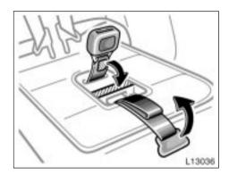
11. To store the built-in child restraint, fasten the shoulder belt clip and return the seat belt buckle using the fastener tapes. Fold up the seat belt adjustment strap (gray tab) in the seat so that the edge of the strap does not come out the raised child restraint seat cushion. Raise the child restraint seat cushion and reinstall the head restraint and upper pad correctly by inserting the posts into the holes.
