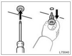
Removing the cover clips (Type A)
