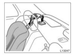
Follow the procedure below for a child restraint system that uses of a top strap to ensure the system. Follow all the installation instructions provided by its manufacturer.
