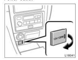
The power outlet is designed for power supply for car accessories.
