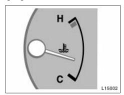
The gauge indicates the engine coolant temperature when the ignition switch is on. The engine operating temperature will vary with changes in weather and engine load.
