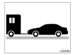
Your vehicle can be dingly towed (with four wheels on the ground) from the front behind a motorhome.
