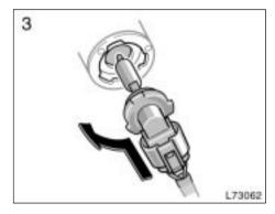
3. Install a new bulb and connector into the mounting hole.
