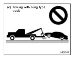
(c) Towing with sling type truck
