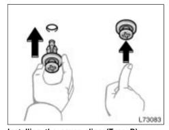
Installing the cover clips (Type B)
