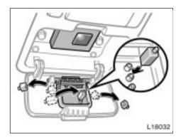
Remove spacers from the center panel. Place the largest spacer on the pin that would be below transmitter button when the cover is closed. Close the cover.
