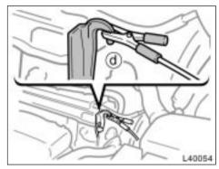
Connecting point for 5S-FE engine
