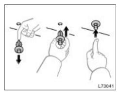
Installing the cover clips (Type A)
