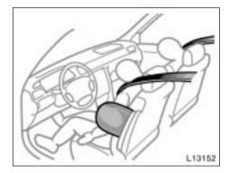
The SRS (Supplemental Restraint System) side airbags are designed to provide further protection for the driver and front passenger in addition to the primary safety protection provided by the seat belts.
