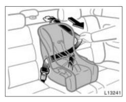
Fully extend the shoulder belt to put it in the lock mode. When the belt is then retracted even slightly, it cannot be extended.
