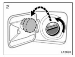
To remove the fuel tank cap, turn the cap slowly counterclockwise, then pause slightly before removing it. After removing the cap, hang it on the cap hanger.
