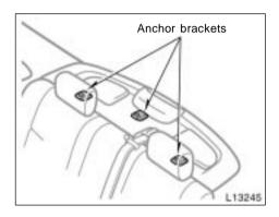
Use the anchor bracket on the package tray behind the rear seat to attach the top strap.
