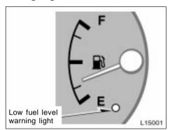
The gauge works when the ignition switch is on and indicates the approximate quantity of fuel remaining in the tank.
