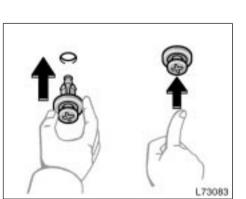
Installing the cover clips
