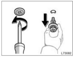
Removing the cover clips (Type B)
