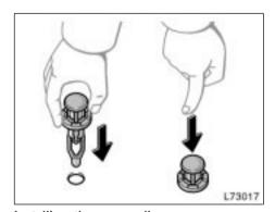
Installing the cover clips
