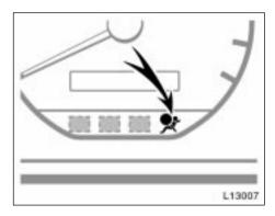
This indicator comes on when the ignition key is turned to the "ACC" or "ON" position. It goes off after about 6 seconds. This means the SRS side airbags are operating properly.
