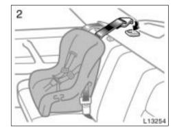
2. Securely fasten the child restraint system with the seat belt.
