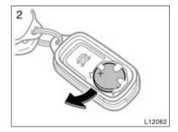
2. Remove the discharged transmitter batterv.
