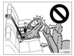
Do not put a rear-facing child restraint system on the rear seat if it interferes with the lock mechanism of the front seats. This can cause severe injury to the child and front passenger in case of sudden braking or a collision.
