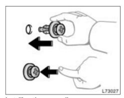
Installing the cover clips
