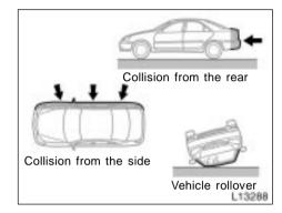
The SRS front airbags are generally not designed to inflate if the vehicle is involved in a side or rear collision, if it rolls over, or if it is involved in a low-speed frontal collision. But, whenever a collision of any type causes sufficient forward deceleration of the vehicle, deployment of the SRS front airbags may occur.
