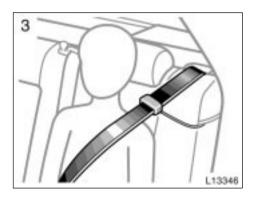
Buckle, position and release the seat belt. (For wearing the seat belt, see "—Fastening front and rear seat belts" on page 46 in this Section.) Make sure the shoulder belt crosses the shoulder.
