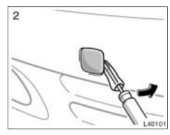
Remove the front towing eyelet cover on the front bumper, using a flatbladed screwdriver which is wrapped with a cloth.
