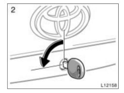
Close the trunk lid. Insert the master key and turn it counterclockwise to deactivate the trunk lid lock release lever.
