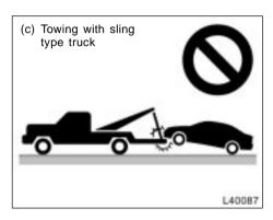
(c) Towing with sling type truck
