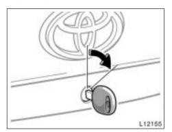
To open the trunk lid from the outside, insert the master key and turn it clockwise.
