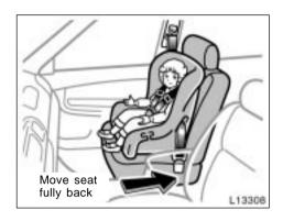
• A forward-facing child restraint system should be allowed to be installed on the front passenger seat only when it is unavoidable. Always move the seat as far back as possible even if the "AIRBAG OFF" indicator light is illuminated, because the front passenger airbag could inflate with considerable speed and force. Otherwise, the child may be killed or seriously injured.
