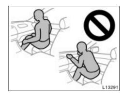
• Do not sit on the edge of the seat or lean against the dashboard when the vehicle is in use, since the front passenger airbag could inflate with considerable speed and force. Anyone who is up against, or very close to, an airbag when it inflates, can be killed or seriously injured. Sit up straight and well back in the seat, and always use your seat belt properly.
