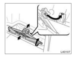
To store the jack, align the hole of the jack head with the vehicle hook. Turn the jack joint until the jack base fits securely with the vehicle body.
