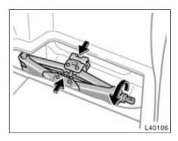
To remove the jack, turn the jack joint by hand until the jack becomes free.
