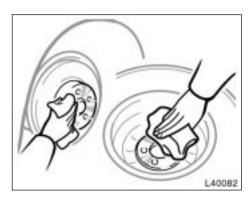
Before putting on wheels, remove any corrosion on the mounting surfaces with a wire brush or such. Installation of wheels without good metal- to- metal contact at the mounting surface can cause wheel nuts to loosen and eventually cause a wheel to come off while driving.
