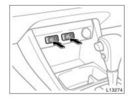
To turn on the seat heater, push the switch. At this time, the indicator light will illuminate to indicate the seat heater is operating.
