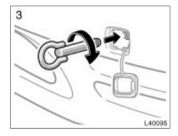
Secure the front towing eyelet to the hole on the bumper by turning clockwise.
