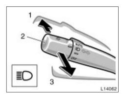
**High-Low beams**—For high beams, turn the headlights on and push the lever away from you (position 1). Pull the lever toward you (position 2) for low beams.
