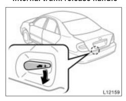
If a person is locked in the trunk, he/she can pull down the phosphorescent handle on the inside of trunk lid to open the trunk lid.
