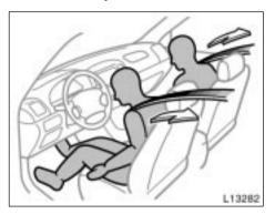
The driver and front passenger seat belt pretensioners are designed to be activated in response to a severe frontal impact.
