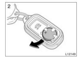
2. Remove the discharged transmitter battery.
