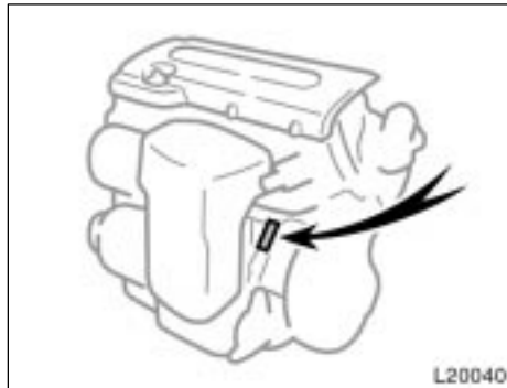
2.4 L 4-cylinder (2AZ- FE) engine
