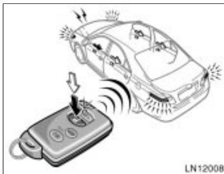
Unlocking operation (vehicles with smart key system)
