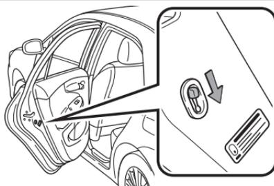
Moving the lever to “LOCK” will allow the door to be opened only from the outside.
