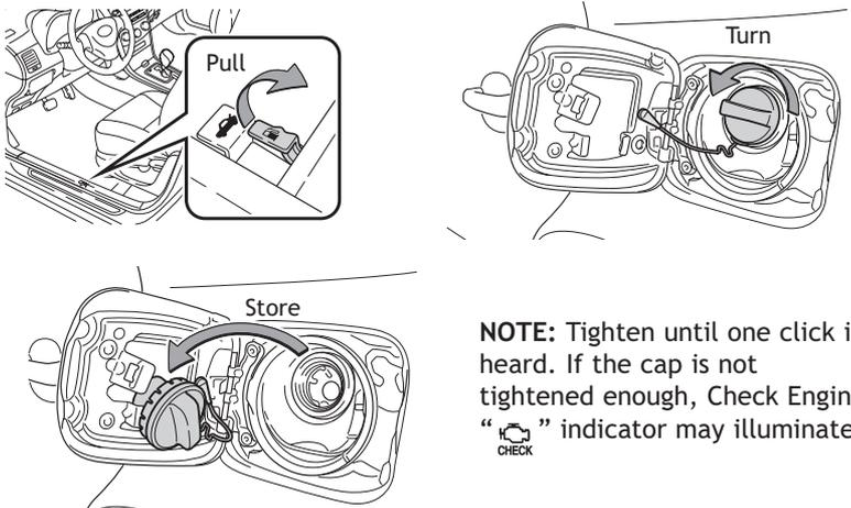
**NOTE:** Tighten until one click is heard. If the cap is not tightened enough, Check Engine “
