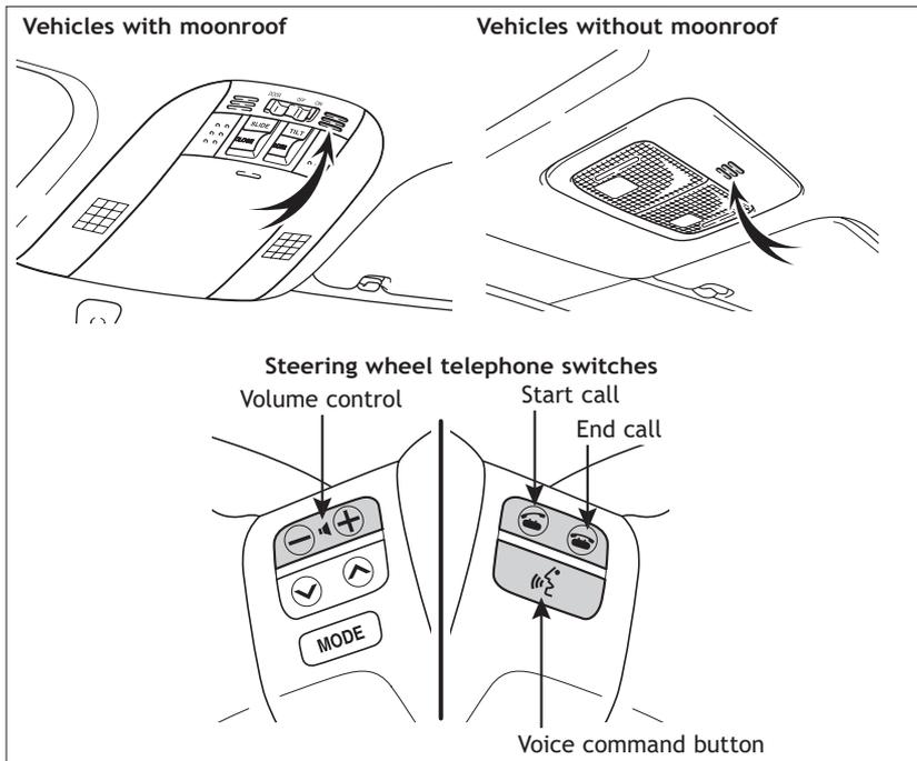
Bluetooth® technology allows you to place or receive calls without taking your hands from the steering wheel or using a cable to connect the compatible telephone and the system.
