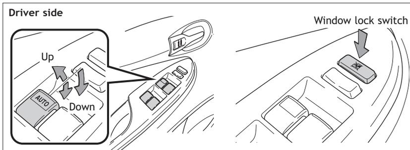
**Automatic operation (driver side only)** Push the switch completely down and release to fully open. To stop window midway, lightly push the switch in the opposite direction.
