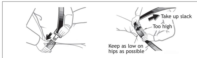
If belt is fully extended, then retracted even slightly, it cannot be re-extended beyond that point, unless fully retracted again. This feature is used to help hold child restraint systems securely.
