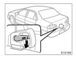
If a person is locked in the trunk, pull down the phosphorescent handle lever on the inside of trunk lid in case of emergency to open the trunk lid.
