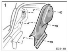
Remove and install the clips as shown in the following illustrations.
