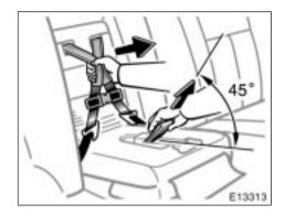
While pulling the seat belt release strap (black), pull both shoulder belts together.
