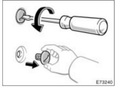
Removing clips (type A): Use a flat-bladed screwdriver or equivalent.
