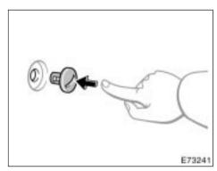
Installing clips (type A)
