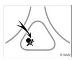
This indicator comes on when the ignition key is turned to the "ACC" or "ON" position. It goes off after about 6 seconds. This means the SRS side airbags are operating properly.
