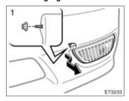
1. Loosen the retainer nut and take out the beam unit.
