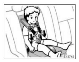
Sit the child on the child seat. Place a shoulder belt over each shoulder. Insert the tabs into the buckle.
