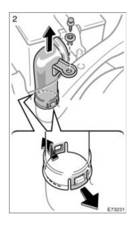
LEFT-HAND HEADLIGHT: Remove the clip and take out the upper cover of the air cleaner duct unit from the lower base as shown in the illustration.
