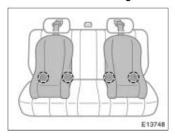
The lower anchorages for the child restraint system interfaced with the FMVSS225 specification are installed in the rear seat.
