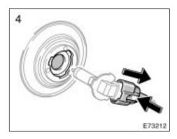
4. Pull the bulb out of the bulb base. Install a new bulb.
