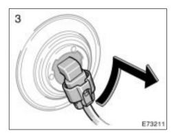
3. Turn the bulb base counterclockwise to the front of the vehicle as shown.
