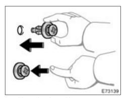
Installing clips (type B)
