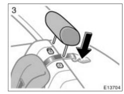
3. Outside anchor brackets only—Replace the head restraint.
