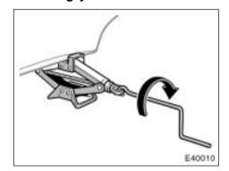
After making sure that no one is in the vehicle, raise it high enough so that the spare tire can be installed.
