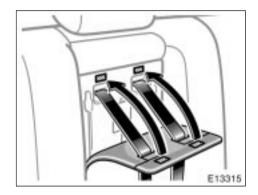
Press the removable pad against the fastener tapes and install the pad to the seatback. Make sure the belts go through the slots in the pad.
