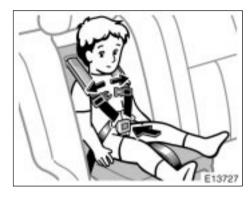
11. To release the child from the seat belts, separate the shoulder belts then press the buckle release button.
