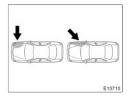
The SRS side airbag system may not inflate if the vehicle is subjected to a collision from the side at certain angles, or a collision to the side of the vehicle body other than the passenger compartment as shown in the illustration.
