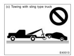
(c) Towing with sling type truck
