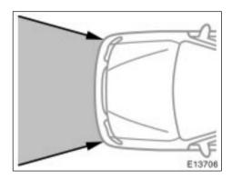
The SRS airbag system is designed to activate in response to a severe frontal impact within the shaded area between the arrows in the illustration.
