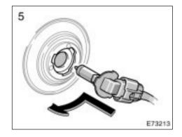
5. Install the bulb base by turning it clockwise to the front of the vehicle.
