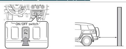
When vehicle is in reverse, a buzzer will sound to inform driver when nearing an obstacle. The system can only be used when the transmission is in the "R" position.
