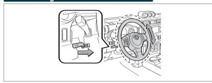
Hold the steering wheel, pull the lock release lever, tilt to the desired angle and release the lever.
