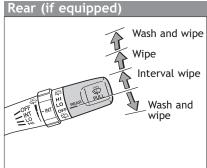
**NOTE:** Rear wiper and washer operate only when back window is fully closed.
