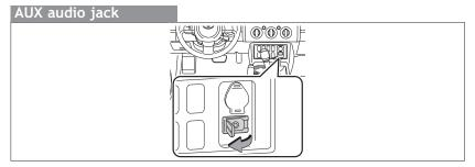
By inserting a mini plug into the AUX audio jack, you can listen to music from a portable audio device through the vehicle's speaker system while in AUX mode.
