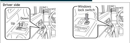
**Automatic down operation (driver side only)** Push the switch completely down and release to fully open. To stop window at any point, lightly pull the switch up.
