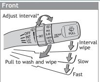
\* Intermittent windshield wiper interval adjustment Rotate to increase/decrease wipe frequency.
