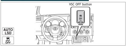
The VSC OFF button is used to switch between modes related to the TRAC, VSC and Auto LSD functions.
