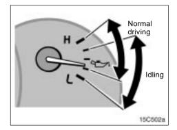
The engine oil pressure gauge indicates engine oil pressure when the ignition switch is on. Check it while driving to make sure the needle is in the proper range.
