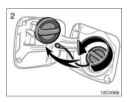
To remove the fuel tank cap, turn the cap slowly counterclockwise, then pause slightly before removing it. After removing the cap, hang it on the cap hanger.
