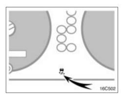
If the vehicle is going to skid during driving, the slip indicator light flashes and an alarm sounds intermittently.
