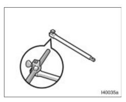
When connecting a jack handle extension with a jack handle end, use a jack handle to tighten the bolts on the joints as shown in the illustration. When connecting the jack handle with extension, tighten the wing bolt on the joint securely. Make sure the hollow meets the bolt on every joint when you tighten the bolts.
