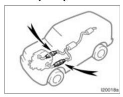
The three-way catalytic converter is the emission control devices installed in the exhaust system.
