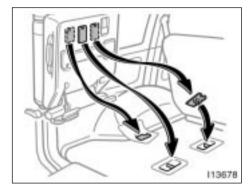
Remove the seat hook covers from the back of the seat cushion, and install them over the seat hooks.
