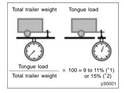
★The trailer cargo load should be distributed so that the tongue load is 9 to 11% for weight carrying hitch (\*1) or 15% for weight distributing hitch (\*2) of the total trailer weight, not exceeding the maximum load of the following:
