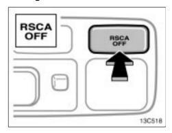
The roll sensing of curtain shield airbags off switch can turn off the curtain shield airbags and front seat belt pretensioners in a vehicle rollover. This switch should only be used in a situation where the inflation is not desired (such as extreme off-road driving).
