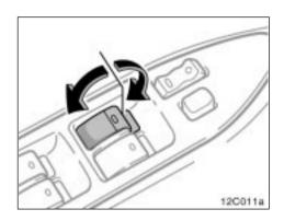
**Automatic operation:** Push the switch completely down or pull it completely up, and then release it. The window will fully open or close. To stop the window partway, lightly move the switch in the opposite direction and then release it.
