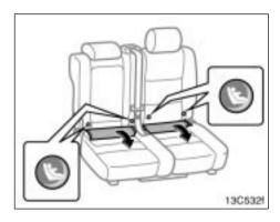
Take off the cover between the seat cushion and seatback and confirm the position of the lower anchorages below the symbol in the seat back.
