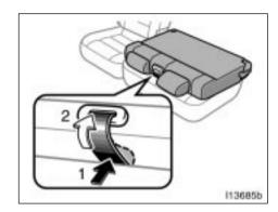
WHEN RETURNING THE SECOND SEAT If you cannot raise the seatback because of the locked seat belt, do not try it hard. Release the lock of the seat belt in the following way. Push in the lower front edge of the seatback cushion to slacken the seat belt (1) and let the seat belt retract a little (2).
