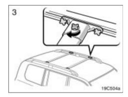
In order to fix the cross rails to the appropriate length, turn the upper knobs clockwise after tightening all of the side knobs.
