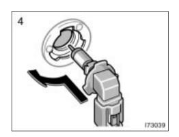
4. Left-hand headlight and right-hand headlight (high beam): Install the bulb base by turning it clockwise to the front of the vehicle. Right-hand headlight (low beam): Install the bulb base by turning it counterclockwise to the front of the vehicle.
