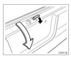
Pull the handle toward you and pull down the lower side of the back door.
