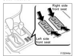
To turn on the seat heater, push the switch to "HI" (high heating temperature) or "LO" (low heating temperature). At this time, the indicator light on either side will illuminate to indicate the seat heater is operating. To turn off the seat heater, push the switch lightly on the opposite side.
