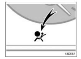
The indicator comes on when the ignition key is turned to the "ON" position. It goes off after about 6 seconds. This means the SRS front airbags are operating properly.
