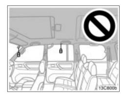
Do not attach a microphone or any other device or object around the area where the curtain shield airbag activates such as on the windshield glass, side door glass, front, center and roof side garnish, roof interior or assist grips. When the curtain shield airbag inflates, the microphone or other device or object will be thrown away with great force or the curtain shield airbag may not activate correctly, resulting in death or serious injury.
