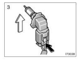
**3. Pull the bulb out of the bulb base.** If the connector is tight, wiggle it.
