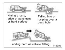
The SRS front airbags may also deploy if a severe impact occurs to the underside of your vehicle. Some examples are shown in the illustration.
