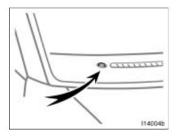
The automatic light control sensor is on the top of the passenger's side instrument panel.
