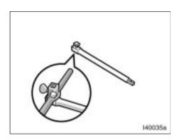
When connecting a jack handle extension with another extension and a jack handle end, use a jack handle to tighten the bolts on the joints as shown in the illustration. When connecting the jack handle with extension, tighten the wing bolt on the jack handle securely. Make sure the hollow meets the bolt on any joint when you tighten the bolts.
