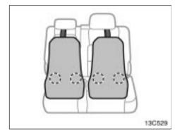
The lower anchorages for the child restraint system interfaced with the FMVSS225 specification are installed in the second seat.
