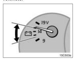
The voltmeter tells whether the battery is charged or discharged. Check it while the engine is running—the needle should always indicate as shown above.
