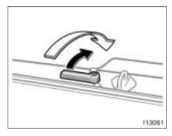
Push the handle and push down the lower side of the back door.
