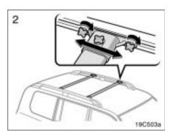
Slide the cross rails to the appropriate position for loading the luggages and turn the side knobs clockwise to tighten the cross rails securely.
