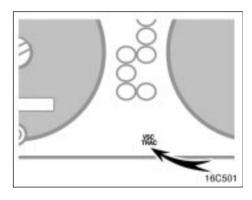
Active traction control system failure warning
