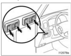
The rear quarter windows can be operated with the "REAR VENT" switches on the instrument panel.
