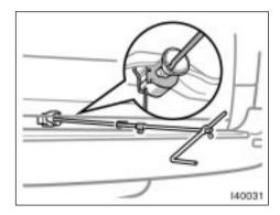
3. Insert the jack handle end into the lowering screw through the access hole and turn it counterclockwise with pushing it to the front lightly.
