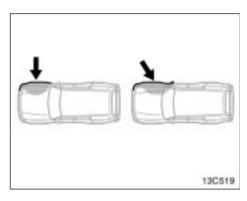
The SRS side airbag and curtain shield airbag system may not activate if the vehicle is subjected to a collision from the side at certain angles, or a collision to the side of the vehicle body other than the passenger compartment as shown in the illustration.
