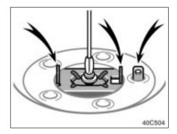
When storing the spare tire, put it in place with the outer side of the wheel facing up and hook the holding bracket as shown in the illustration. Then secure the tire, taking care that the tire goes straight up without catching on any other part, to prevent it from moving during a collision or sudden braking.
