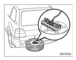
4. After the tire is lowered completely to the ground, remove the holding bracket as shown in the illustration.
