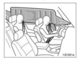
The SRS (Supplemental Restraint System) side airbags and curtain shield airbags are designed to provide further protection for the driver, front passenger and second seat passengers in addition to the primary safety protection provided by the seat belts.
