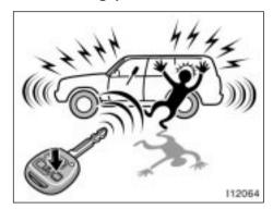
Pushing the "PANIC" switch for 1 second blows the horn intermittently and flashes the headlights, tail lights and interior lights.\*
