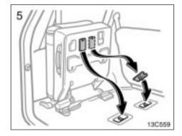
Remove the seat hook covers from the back of the seat cushion, and install them over the seat hooks.
