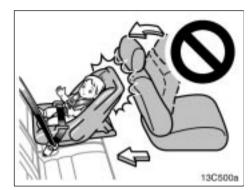
Child restraint systems installed on the third seat should not contact the second seatbacks.
