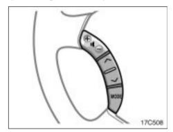
The switches are installed on the left side of the steering wheel.
