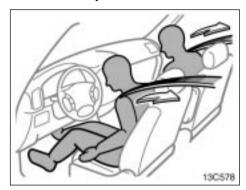
The driver and front passenger seat belt pretensioners are designed to be activated in response to a severe frontal impact or a vehicle rollover.
