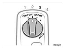
This skyhook TEMS adjusts the damping effect on the shock absorbers with the damping mode select switch. Select one of the 4 modes which is suited to the driving conditions with the damping mode select switch to provide good riding comfort and stability.
