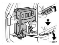
After tumbling the third seat, open the cover, hold the whole seat and pull it up while pulling the handle toward you.
