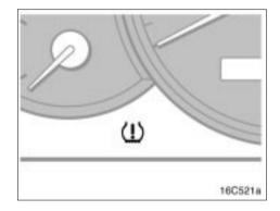
The tire pressure warning light comes on when the ignition switch is turned to the "ON" position and goes off after a few seconds. This means the tire pressure warning light is operating properly. If the tire inflation pressure becomes low, the light comes on again. In this case, adjusting the tire inflation pressure will turn off the light after a few minutes. If the light blinks, the tire pressure warning system is not working properly.
