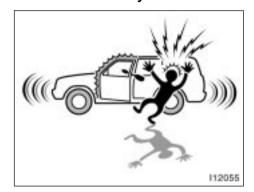
To deter vehicle theft, the system is designed to sound an alarm if any of the side doors, back door or hood is forcibly unlocked or opened or the battery terminal is disconnected and then reconnected when the vehicle is locked.
