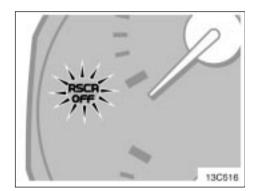
Make sure the roll sensing of curtain shield airbags off indicator is not on. The curtain shield airbags will not inflate in a vehicle rollover if this indicator light is on and you may be killed or seriously injured.
