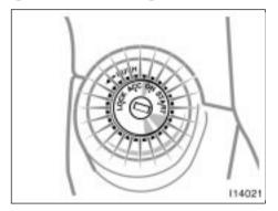
For easy access to the ignition switch, the ignition switch light comes on when any door is opened.
