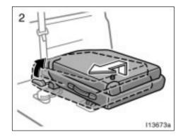
Unlock the seat cushion and slide the whole seat to the rear-most position while pulling up the handle.
