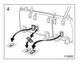
Remove the seat hook covers from the back of the seat cushion, and install them over the seat hooks.
