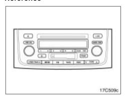
AM·FM radio/cassette player/compact disc changer controller/compact disc player with changer (with XM® satellite radio\* controller)
