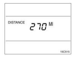
**▼**Driving distance after engine starting The driving distance after engine starting is displayed.
