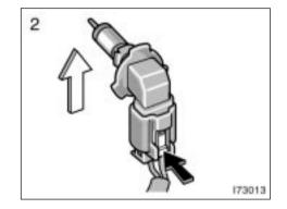
**2. Pull the bulb out of the bulb base.** If the connector is tight, wiggle it.
