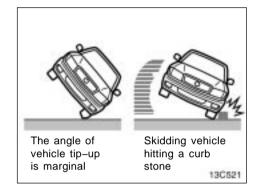
The curtain shield airbags may inflate if the angle of vehicle tip-up is marginal or if the skidding vehicle's tires hit a curb stone laterally as shown in the illustration.
