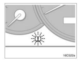
If the tire pressure warning light does not blink slowly three times when you push and hold the reset switch, initialization has failed and the tire pressure warning system may not work properly. In this case, initialize the system again. If initialization cannot be performed, have the system checked at your Toyota dealer.
