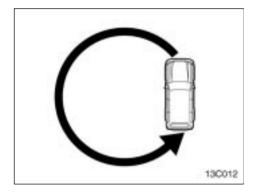
Drive the vehicle slowly (at 8km/h (5mph) or lower) in a circle until the direction is displayed. If there is not enough space to drive in a circle, drive around the block until the direction is displayed.
