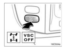
Pushing the center differential lock button automatically turns the vehicle stability control system off. At this time, the "VSC OFF" indicator comes on with the center differential lock indicator light. (For details, see "Four-wheel drive system—(a)Four-wheel drive control" on page 149.)
