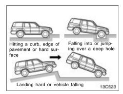
The SRS side airbags and curtain shield airbags may deploy if a severe impact occurs to the underside of your vehicle. Some examples are shown in the illustration.
