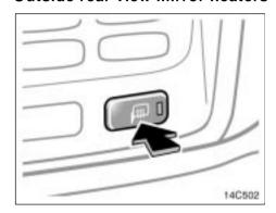
To defog or defrost the outside rear view mirrors, push the switch.
