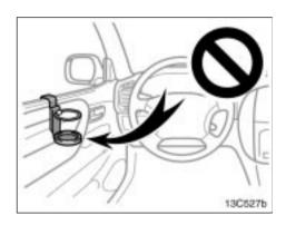
Do not attach a cup holder or any other device or object on or around the door. When the side airbag inflates, the cup holder or any other device or object will be thrown with great force, or the side airbags may not activate correctly, resulting in death or serious injury. Likewise, the driver and front passenger should not hold objects in their arms or on their knees.
