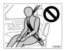
Do not allow anyone to lean against the door when the vehicle is in use, since the side airbag and curtain shield airbag could inflate with considerable speed and force. Otherwise, he/she may be killed or seriously injured. Special care should be taken especially when you have a small child in the vehicle.
