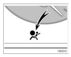
The indicator comes on when the ignition key is turned to the "ON" position. It goes off after about 6 seconds. This means the SRS side airbags and curtain shield airbags are operating properly.
