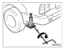
After making sure no one is in the vehicle, raise it high enough so that the spare tire can be installed.
