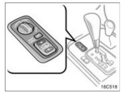
This active height control suspension controls the vehicle height depending on the vehicle driving condition. Select your desired height among the "HI" (high), "N" (normal) and "LO" (low) modes with the height select switch.
