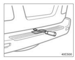
2. Remove the access hole cover on the rear bumper with a flathead screwdriver.
