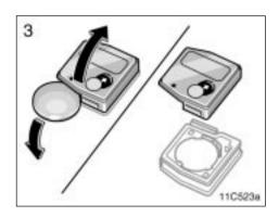
Open and remove the battery case cover using a coin. Remove the discharged battery and put in a new battery with the positive side up.
