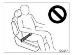
Vif the seat belt extender has been connected to the driver's seat belt buckle without the driver actually wearing the seat belt, the SRS driver's airbag system will judge that the driver is wearing it. In this case, the driver's airbag may not activate correctly, causing death or serious injury in the event of collision. Be sure to wear the seat belt with the seat belt extender.
