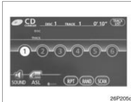
(c) Selecting a desired disc (Type 1 only) Touch the desired disc number.
