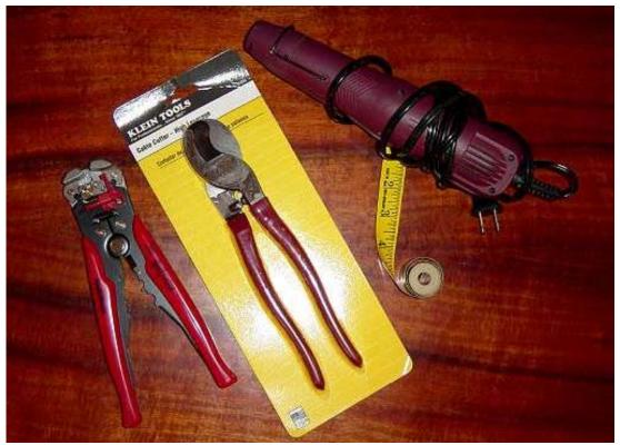
Here is a picture of some of the tools you may need to do the job. Wire cutters are very useful for cutting through the thick 4 gauge wires, measuring tape is useful for measuring the custom lengths of wires that you will need. The heat gun for shrinking the heat shrink tubing. On the left is a wire stripper/crimper tool, but that one pictured does not do a good job for crimping 4 gauge connectors.
