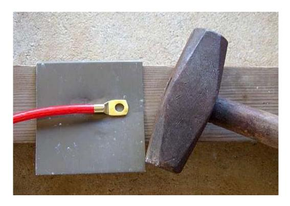
Unless you have a professional grade wire crimper, your best way to crimp these 4 gauge wire terminals is with a huge 10 lb. Hammer/mallet. Believe me, this works the best. Give it a few heavy hits until the terminal is tight onto the wire.
