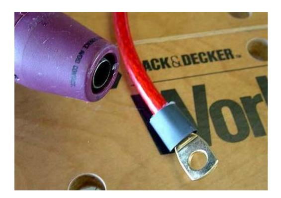
Cut some heat shrink tubing to fit around the siliconed area, and use a heat gun or hair dryer to shrink the tube into place. The gold plated connectors come with a plastic housing, you can slip them into place.
