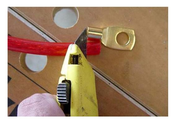
Cut the insulation surrounding the wire that matches with the wire connector housing. A utility knife works well.
