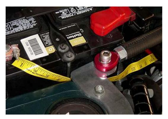
The first step is to measure from point A to point B how much wire is needed to go between each location. This is how much wire you will cut off from your 9 feet of wire. Make sure that you allow enough space for the wire connectors on each end.
