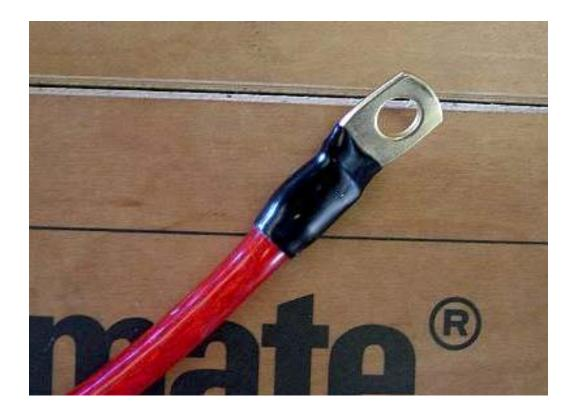
This is what the finished end should look like. Repeat on the opposite side, and you will have made a custom ground wire. Just a note, depending on the size of the hole in your connector, you may have to drill it out bigger to fit some of the attaching bolts.
