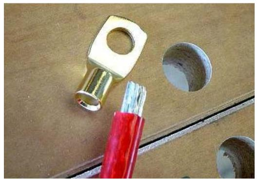
This is what the wire end will look like once you cut off the insulating material. Slide the wire connector over the exposed wire and get ready to crimp it.
