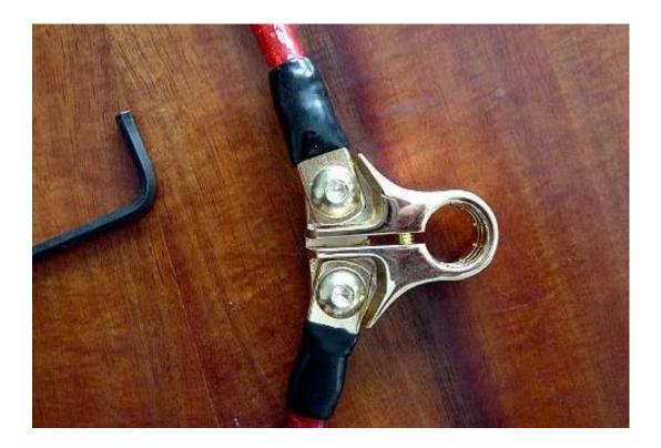
Here is what it looks like on the bottom of the negative battery terminal. You can screw on 2 wire terminals on either end with an Allen wrench.
