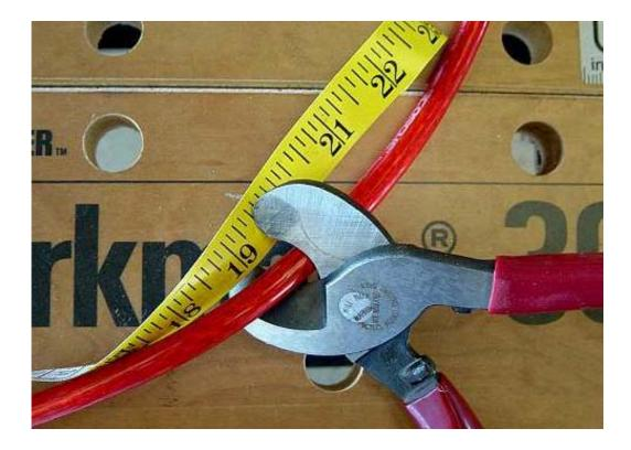
Next, you need to measure the length of wire that you need and cut it with the wire cutters. This type of cutter shown above will cut the 4 gauge insulated wire with ease.
