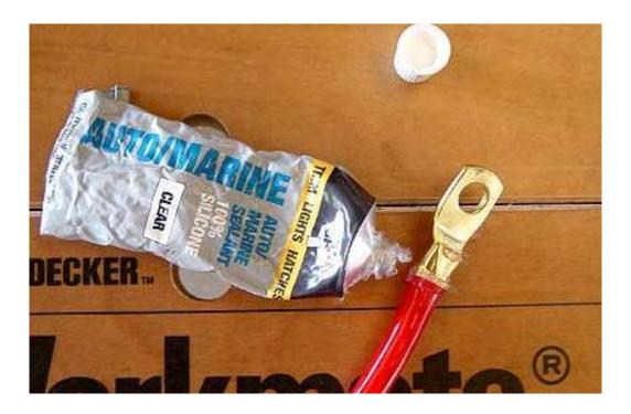
Apply some silicone sealant around the edges where the terminal and wire sleeve meet. You do not want any moisture to seep in and corrode the copper wires, so be generous with the sealant.
