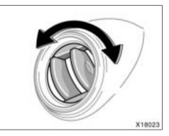
You can change air flow direction by turning the side vents.
