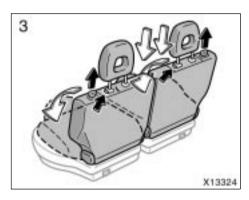
3. Lower the head restraint to the lowest position. Pull up the strap to unlock the seatback and fold the seatback forward until it locks.
