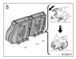
5. Make sure the front legs are locked and the seat is securely locked in position.
