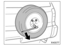
2. Turn the hold-down nuts counterclockwise with the wheel nut wrench and remove them.
