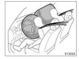
The SRS (Supplemental Restraint System) airbags are designed to provide further protection for the driver and front passenger in addition to the primary safety protection provided by the seat belts.
