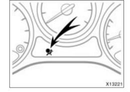
This indicator comes on when the ignition key is turned to the "ON" position. It goes off after about 6 seconds. This means the front seat belt pretensioners are operating properly.
