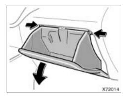
1. Push each side of the glove box to disconnect the claws.
