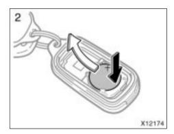
2. Remove the discharged transmitter battery.
