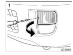
1. Loosen the retainer screw with a Phillips-head screwdriver and take out the front turn signal light unit.
