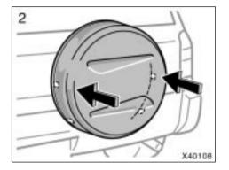
2. Push both sides of the cover and set the cover by hooking the 4 inside protrusions.
