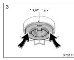
3. Install the rubber cover with the "TOP" mark upward, and fit it securely on the boss. Plug in the connector.
