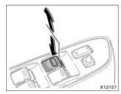
Automatic operation: Push the switch completely down or pull it completely up, and then release it. The window will fully open or close. To stop the window partway, lightly move the switch in the opposite direction and then release it. Jam protection function: During automatic closing operation, the window stops and opens half way if something gets caught between the window and window frame.
