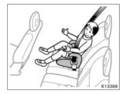
(C) BOOSTER SEAT INSTALLATION A booster seat is used in forward-facing position only.
