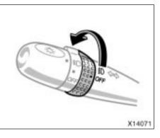
To turn on the front fog lights, twist the band of the headlight and turn signal switch lever. They will come on only when the headlights are on low beam. Interior lights
