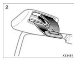
2. Insert the round end tab into the cover. You will hear a click when the tabs are locked in the seat belt cover. Make sure the tabs are securely locked in the cover.
