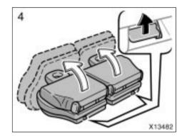
4. Pull up the seat cushion lock release lever and swing the whole seat up and forward.
