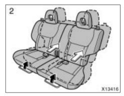
2. Hold the center of the lever and pull it up. Then slide the rear seat fully backward and pull it forward slightly till it locks.
