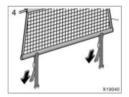
4. Pull the end of the belt to stretch the net securely.
