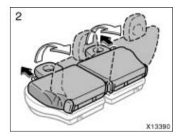
2. Pull the seatback lock release strap and swing the seatback up.
