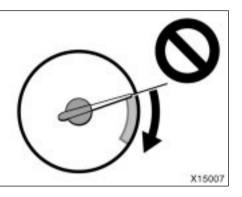
The tachometer indicates engine speed in thousands of rpm<sup>2</sup>(revolutions per minute). Use it while driving to select correct shift points and to prevent engine lugging and over-revving.
