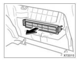
2. Remove the filter case from the filter outlet as shown in the illustration.
