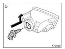
5. Install a new bulb and the connector into the mounting hole. Install the front fog light unit then the front turn signal light unit, and tighten the retainer screw.
