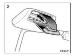
2. Insert the round end tab into the cover. You will hear a click when the tabs are locked in the seat belt cover. Make sure the tabs are securely locked in the cover.
