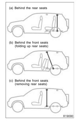
You can separate the luggage compartment by installing the separation net. You can choose one of the three positions.
