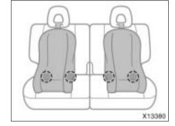
The lower anchorages for the child restraint system interfaced with the FMVSS225 specification are installed in the rear seat.
