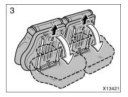
3. To unlock the seat, hold the upper back of the seat with your hand and pull the lock release strap up. Swing the whole seat down and set the rear legs to the hooks on the floor. Make sure the rear legs are securely set to the hooks by trying to pull up the rear part of the seat.
