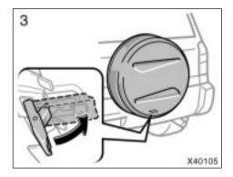
3. Lock the latch handle which is on the bottom of the cover.
