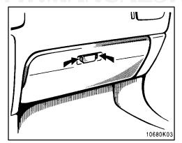
To open the glovebox door, compress the lock release buttons.
