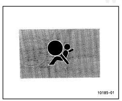
This SRS airbag system has a service reminder indicator to inform the driver of operating problems. If either of the following conditions occurs, this indicates a malfunction of the airbag. Contact your Toyota dealer as soon as possible to service the vehicle.
