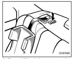
4. If your child restraint system requires the use of a top strap, latch the hook onto the anchor bracket and tighten the top strap.
