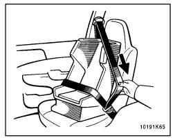
2. Fully extend the shoulder belt to put in the lock mode.
