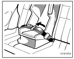
2. Make sure the belt is tight by pulling its free end while you firmly push down the child restraint system.
