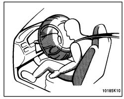
The SRS (Supplemental Restraint System) airbag is designed to provide further protection to the driver when added to the primary protection provided by the seat belt.
