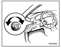
To adjust the brightness of the instrument panel lights, turn the knob.
