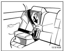
2. Fully extend the shoulder belt to put it in the lock mode.
