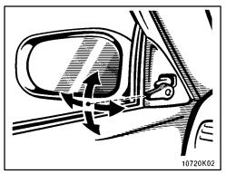
To adjust the rear view mirror, simply operate the control lever.
