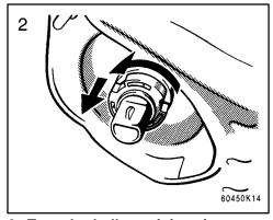
2. Turn the bulb retaining ring counterclockwise and take out the bulb.
