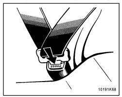
4. To remove the child restraint system, press the buckle-release button and allow the belt to retract.
