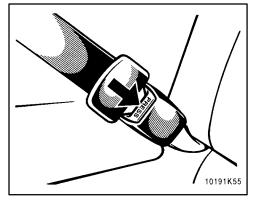
4. To remove the child restraint system, press the buckle-release button and unhook the top strap.
