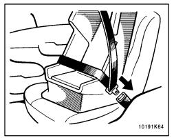
1. Fasten the lap and shoulder belt over the child restraint system following the instructions provided by its manufacturer. Keep the lap portion of the belt tight.
