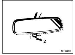
To reduce glare from the headlights of the vehicle behind you during night driving, operate the lever on the lower edge of the mirror.
