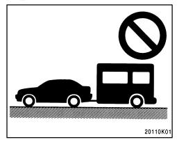
Toyota does not recommend towing a trailer with your Tercel. It is not designed for trailer towing.
