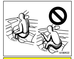
Do not sit on the edge of the seat or lean over the dashboard when the vehicle is in use. The airbags inflate with considerable speed and force; you may be severely injured. Sit up straight and well back in the seat, and always use your seat belt.
