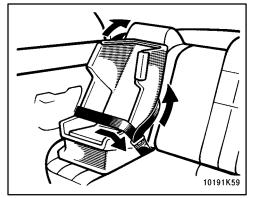
3. Place the shoulder belt between the vehicle seatback and the child restraint system and allow it to retract. To hold the child restraint system securely, let the shoulder belt retract as far as it will go while firmly pushing down the child restraint system.
