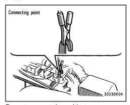
Do not connect the cable to or near any part that moves when the engine is cranked.
