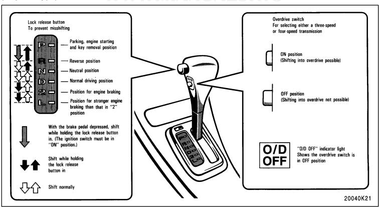
Your automatic transmission has a shift lock system to minimize the possibility of incorrect operation. This means you can only shift out of "P" position when the brake pedal is depressed (with the ignition switch in "ON" position and the lock release button depressed).
