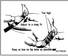
Remove excess length of the belt and adjust the belt position.
