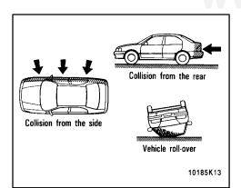
The SRS airbag is not designed to inflate if the vehicle is subjected to a side or rear impact, if it rolls over, or if it is involved in a low-speed frontal collision.
