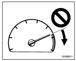
The tachometer indicates engine speed in thousands of rpm (revolutions per minute). Use it while driving to select correct shift points and to prevent engine lugging and overreving.
