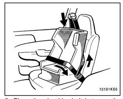
3. Place the shoulder belt between the vehicle seatback and the child restraint system and allow it to retract. To hold the child restraint system securely, let the shoulder belt retract as far as it will go while firmly pushing down the child restraint system.
