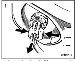
1. Open the hood. Disconnect the connector while depressing the lock release.
