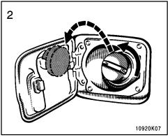
2. To remove the fuel tank cap, turn the cap slowly counterclockwise, then pause slightly before removing it. After removing the cap, hang it on the cap hanger.
