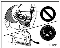
• Do not use a rear-facing child restraint system in the front seat because the force of the rapid inflation of the passenger airbag may cause severe injury to the child. Vehicles with a passenger airbag display a caution label on the passenger side instrument panel as shown above to remind you not to install a rear-facing child restraint system on the front seat.
