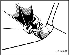
5. To remove the child restraint system, press the buckle-release button and allow the belt to retract. Unhook the top strap.
