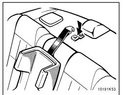
3. If your child restraint system requires the use of a top strap, latch the hook onto the anchor bracket and tighten the top strap.
