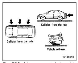
The SRS airbags are not designed to inflate if the vehicle is subjected to a side or rear impact, if it rolls over, or if it is involved in a low-speed frontal collision.
