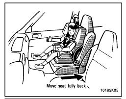
• When using a forward-facing child restraint system in the front seat, the seat must be moved as far back as possible. For instructions concerning the installation of a child restraint system, see "Child restraint" in this chapter.
