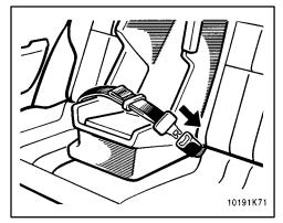
1. Fasten the center lap belt over the child restraint system following the instructions provided by its manufacturer.
